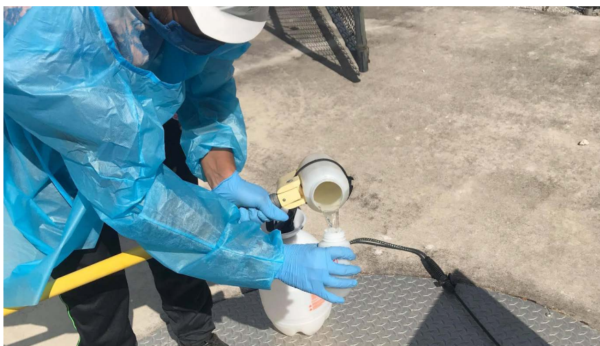
Figure 2. Sample collection from a representative lift station.
