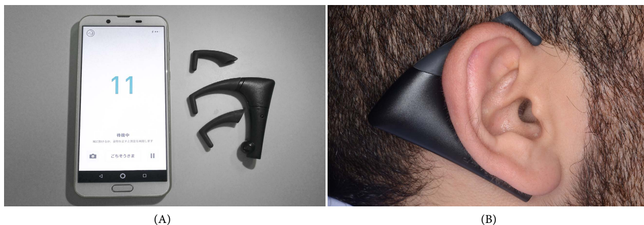
Figure 2. Bitescan system. (A) Bitescan is connected to a smartphone via Bluetooth; (B) Bitescan in position.
