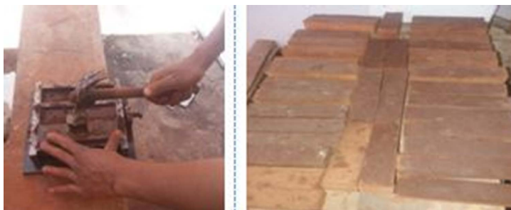
Figure 9. Compaction test and maturation in ambient air.
