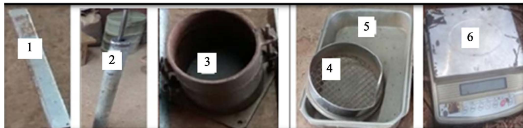
Figure 3. Materials for the proctor test: 1. Razor blade; 2. Proctor rammer; 3. Proctor mold; 4. 20 mm diameter sieve; 5. Tray; 6. Balance.
