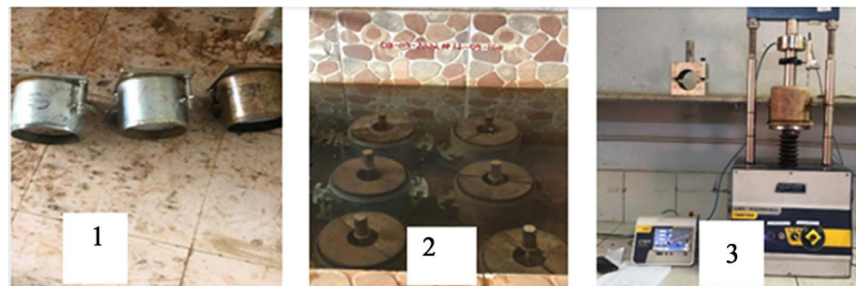
Figure 4. Equipment for the CBR test 1: CBR mold; 2: Water tank; 3: CBR press.
