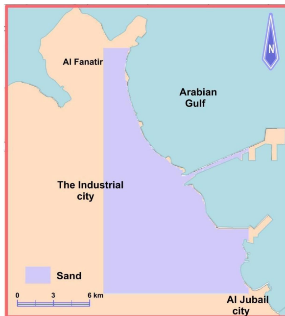
Figure 9. This map identifies surface and near-surface soil types—primarily poorly graded sand (SP) and silty sand (SP-SM). It delineates early foundation zones that require densification or replacement before construction.
