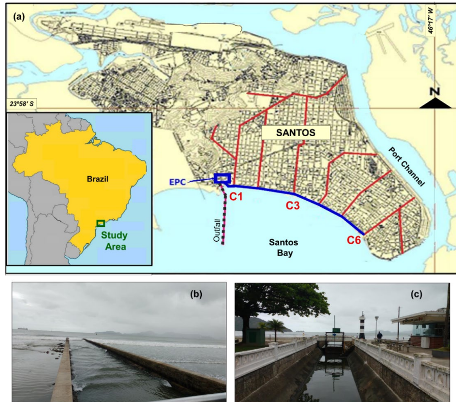
Figure 2. (a) Santos City localization and its integrated system of freshwater runoff capitation. The network of pluvial canals is shown in red, highlighting the sampling locations in canals 1, 3, and 6. In blue, it shows the integration between pluvial canals and the sewage treatment system, where the water flow is directed to the Sewage Preconditioning Station (EPC) and, subsequently, released by the submarine outfall. Details of the external (b) and internal (c) sides of an operating gate.
