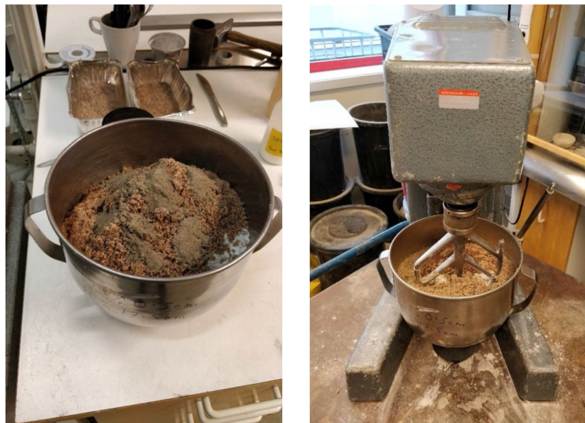
Figure 3. Hobart mixer used to prepare the grout material.
