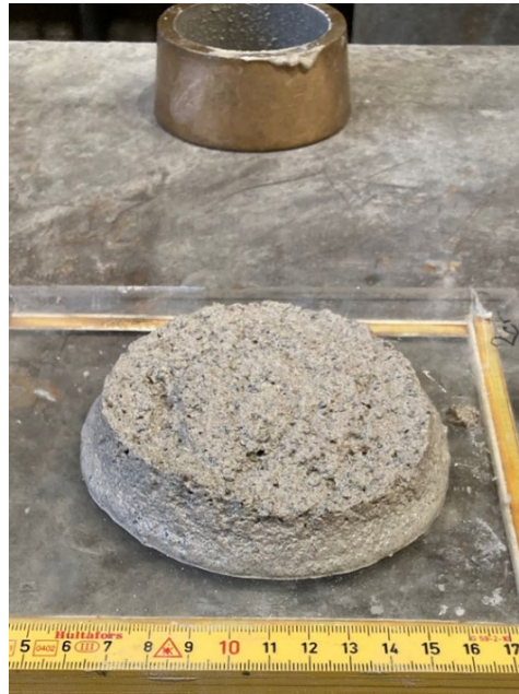
Figure 2. Mini-slump flow test. Bottom diameter of the grout material is ~100 mm (Lagerlund et al., 2023).
