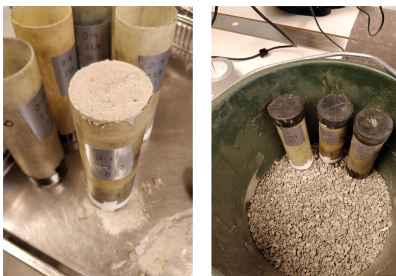
Figure 4. Preparation of samples of LMG material for storage.
