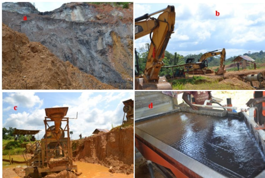
Figure 2. (a) Open Pit at the Mine; (b) Excavators used at the Mine; (c) Hammer Mill used at the Mine; (d) Shaking Table used at the Mine.
