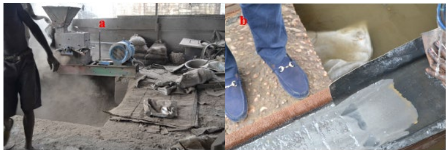
Figure 3. (a) Disc Mill in use; (b) Washing of Ore on a Sluice Box.
