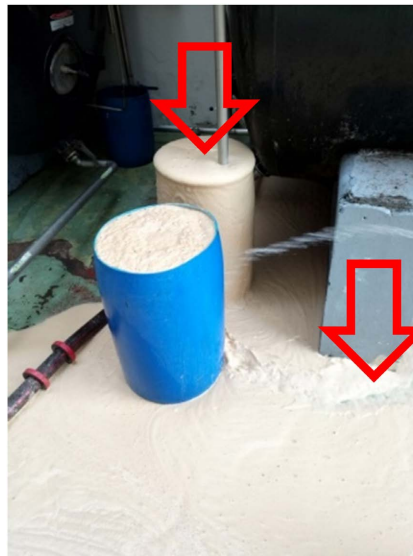
Figure 3. An incident occurred during the transfer of the yeast to the various thermolysis tanks. The red arrow indicates a deposit of spent grain around the rainwater pipe.
