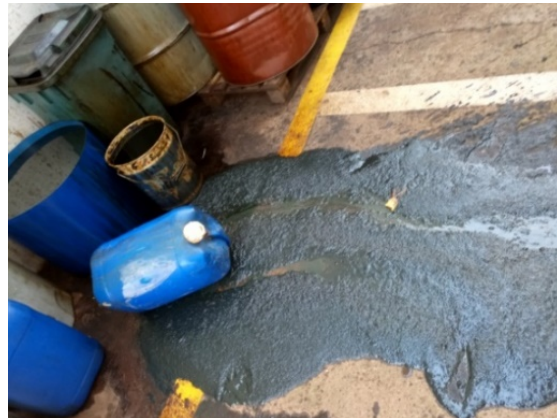
Figure 5. Case of spillage of used oil from a container still containing the remains of chemicals.
