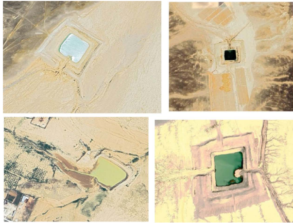
Figure 3. The images illustrate examples of rainwater harvesting ponds utilized in Jordan. Most of these ponds are characterized by a square design, with a side length reaching approximately 150 meters, and a storage capacity of up to 100,000 cubic meters. However, many of these ponds require near-annual rehabilitation due to slope failures and sediment accumulation, which diminish their effective storage capacity.
