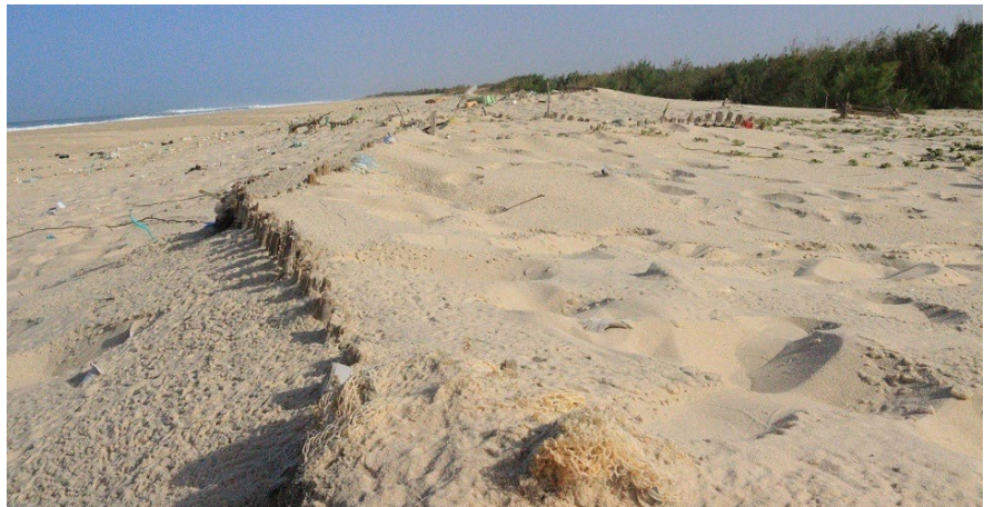
Figure 13. Image showing “Typhavelles” traps filled with sediment.
