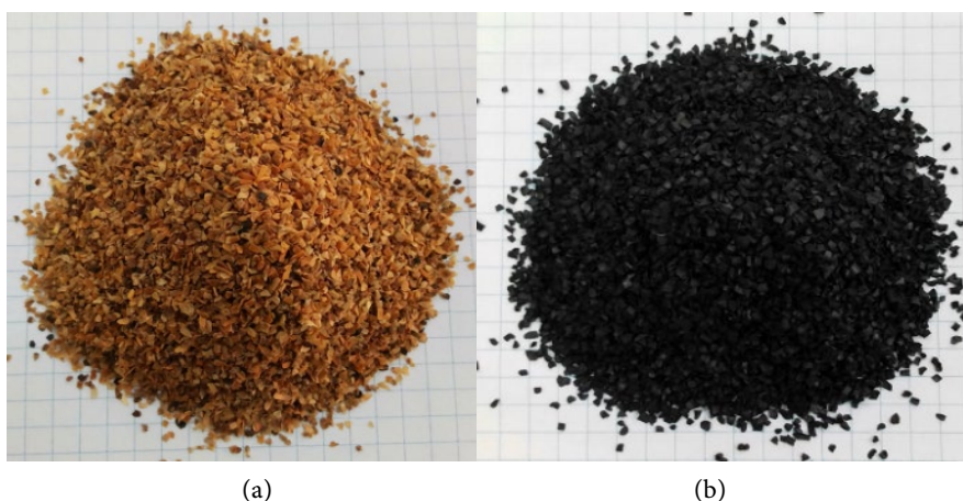
Figure 1. (a) Neem seed cakes after washing; (b) Activated carbon obtained from neem cake.
