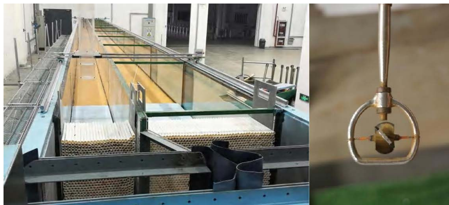
Figure 1. Flume and propeller current meter.
