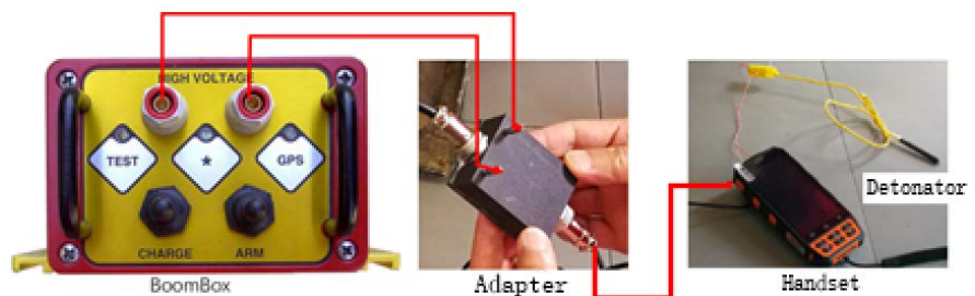
Figure 3. Connection diagram of type A electronic detonator initiation system.
