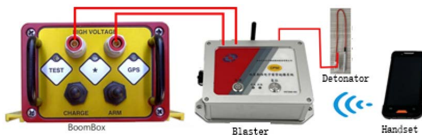
Figure 4. Schematic diagram of connection of B-type electronic detonator initiation system.
