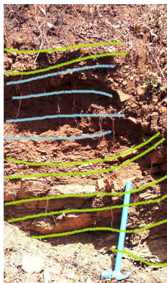
Figure 7. Soil profile with alteration of bedrock Mica schist and Quartzite. The green line indicates patches of Quartzite, and the green line indicates patches of Mica schist.
