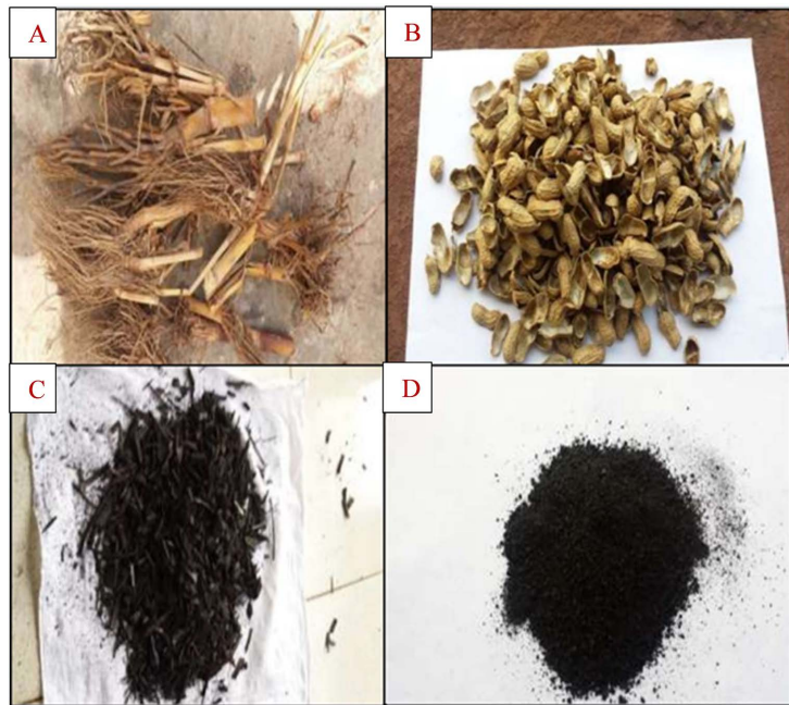
Figure 1. Biomass feedstocks used as raw materials: (A) Millet Stock; (B) Groundnut shells; (C) Charred millet; (D) Commercially sourced anthracite.
