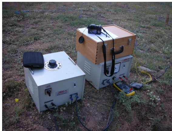
Figure 8. High voltage and high current capacity direct current geophysical device used in this study.
