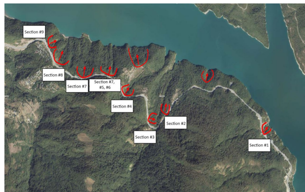
Figure 3. Landslide areas on the right slope of the Zhinvali Reservoir.
