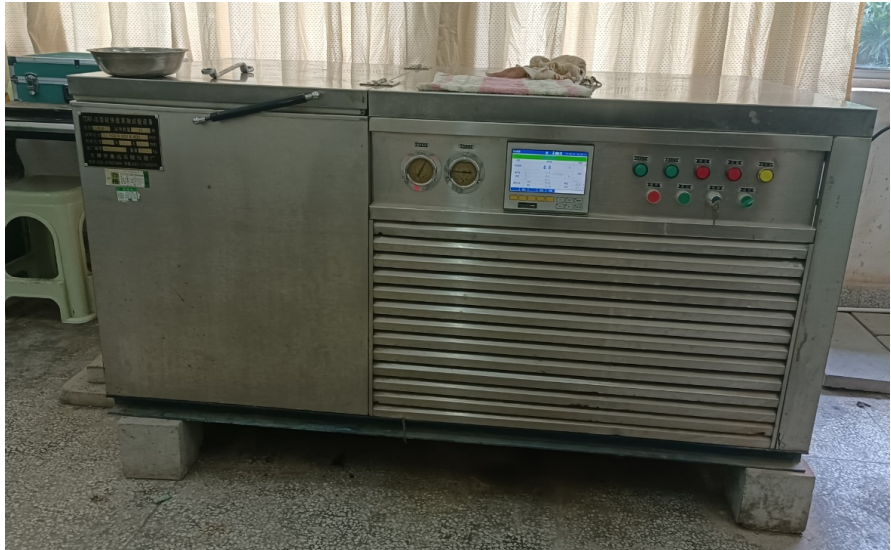
Figure 3. The freeze-thaw testing machine used in the experiment.
