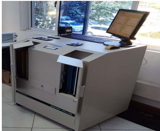
Figure 3. Harshaw 8800 TLD reader system.
