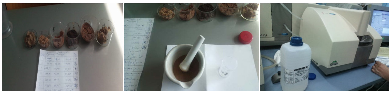
Figure 7. Dried sample from the Oven (left), crushed to separate particles (middle) and the Malvern Instruments Mastersizer 2000 Measuring unit used for diffusion laser granulometry (right).
