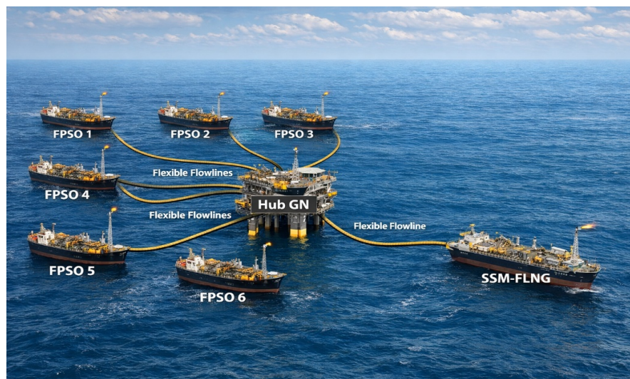
Figure 1. Representation of the hub platform receiving natural gas from various FPSOs and delivering it to SSM-FLNG.
