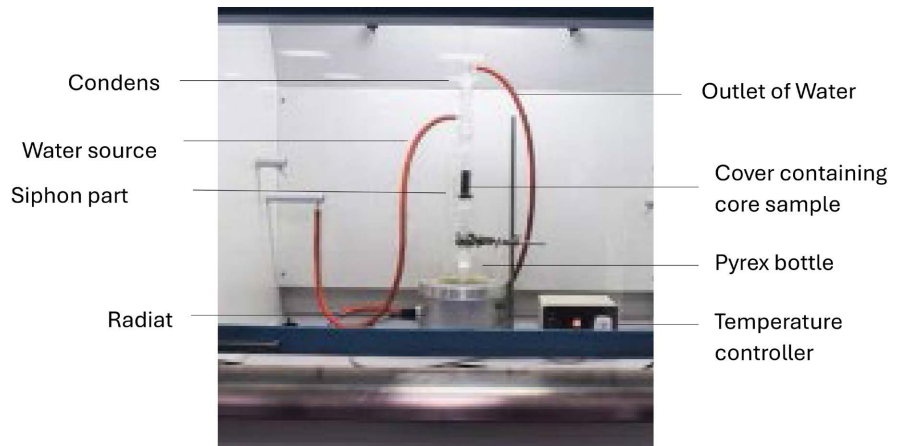
Figure 6. Soxhlet extractor to clean the core samples.
