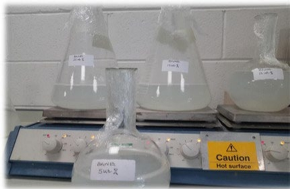
Figure 2. Mixing silica and AG with brine contained (5 wt%, 10 wt%, 15 wt% and 20 wt%).
