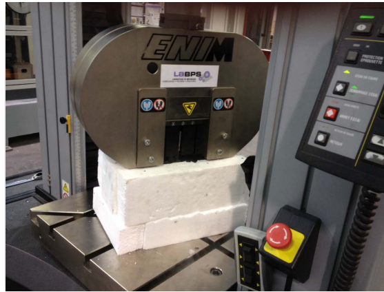
Figure 7. Nitrogen tank insulated with 50 mm thick polystyrene panels.
