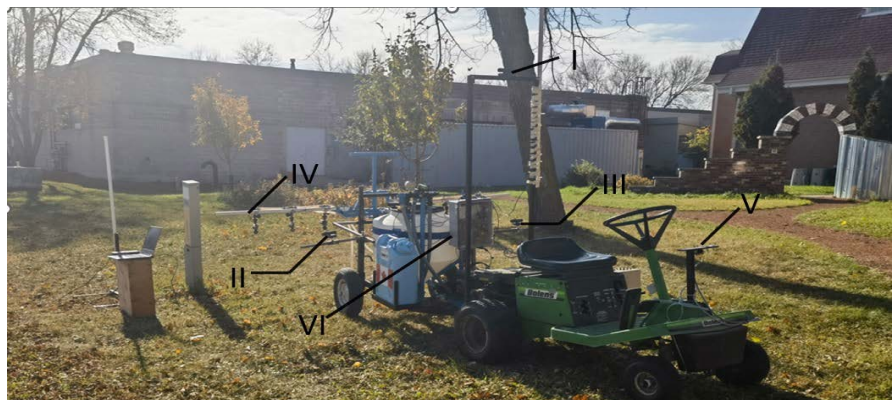
I-Front Camera, II-Right Camera, III-Left Camera, IV-Nozzle with Solenoid valve, Control Boom, VI-Electric Box.
