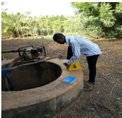
Figure 3. Piezometric measurement in a well with a piezometric probe.
