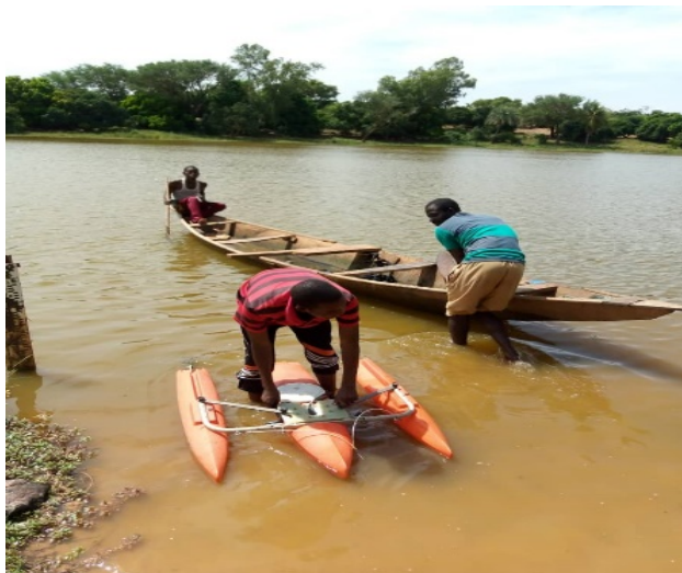
Figure 4. Bathymetric measurement with an ADCP in Bangou bi.
