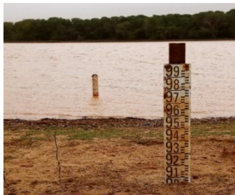
Figure 2. Limnometric scales in Bangou Kirey for water level measurement.
