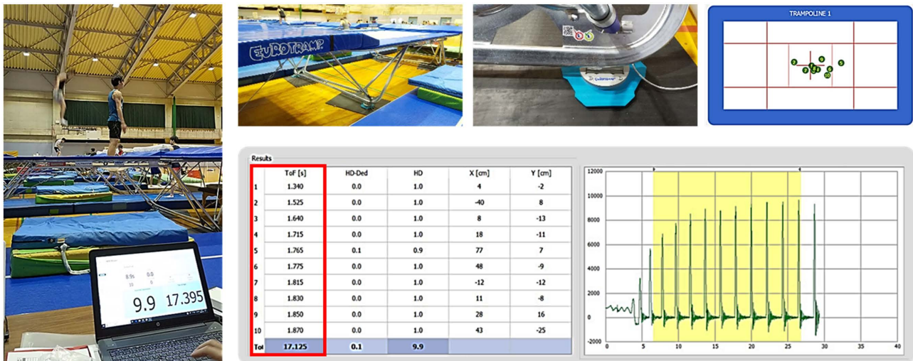
Figure 3. Measurement of flight time, using an all-in-one measurement system (HDTs EU-7100). The red squares indicate the flight time of each jump, and the total flight time of the 10 jumps is shown at the bottom.
