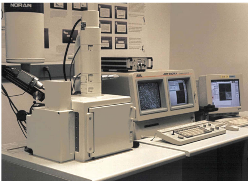
Figure 3. In scanning electron microscopy (SEM), fast electrons interact with solid samples, generating various signals such as secondary electrons (SEM image), backscattered electrons (BSE), and characteristic X-rays.
