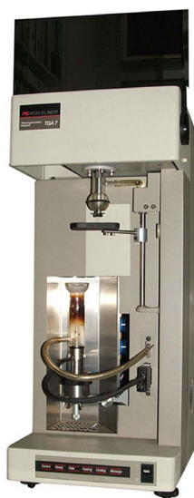
Figure 4. Thermogravimetric Analysis (TGA) measures sample mass changes over temperature, offering insights into physical and chemical phenomena, especially useful for polymer analysis.
