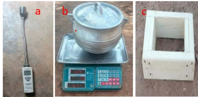
Figure 1. a) Digital thermometer, b) Digital scale, c) Wooden mold measuring 30 \times 14 \text{ cm} \times 10 \text{ cm} .
