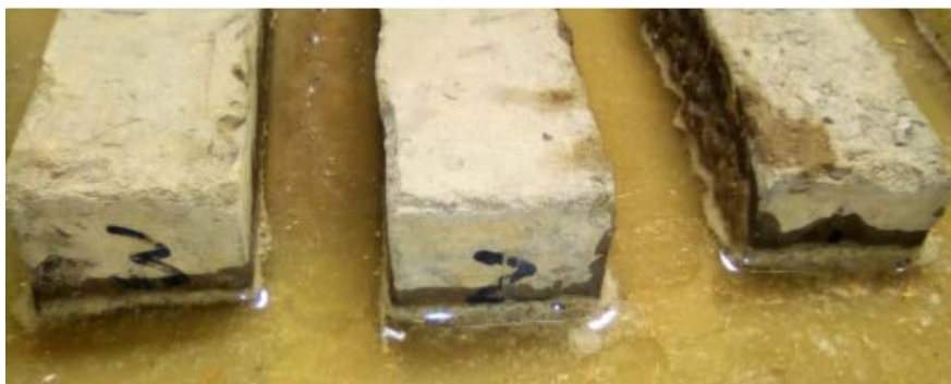
Figure 4. Water absorption test by capillarity of adobes.
