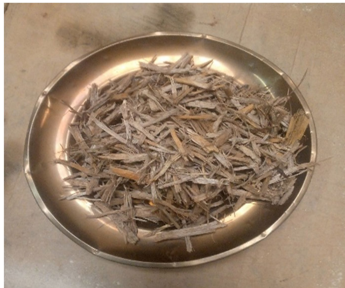
Figure 2. Unscreened sugarcane bagasse fiber from Saris Congo after extraction at the factory.
