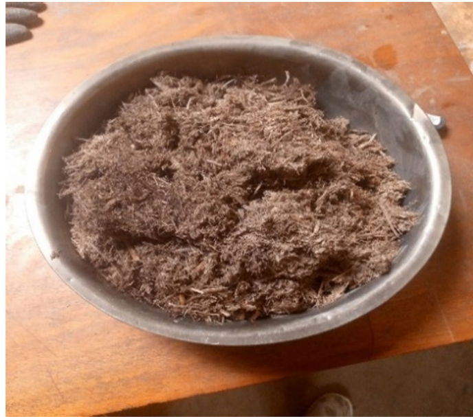
Figure 1. Sieved sugarcane bagasse fiber.
