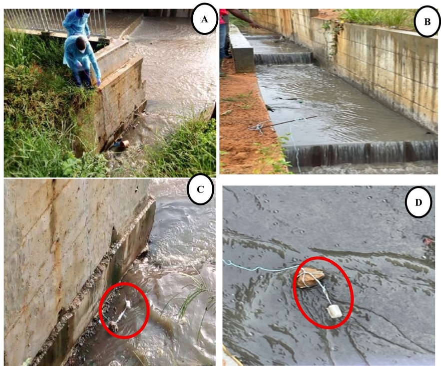
Figure 2. Wastewater monitoring sites in Côte d'Ivoire [19] (A: Grab sampling; B: Open channel for the drainage of water from households; C and D: Passive sampling with sanitary tampon tied to a rope).
