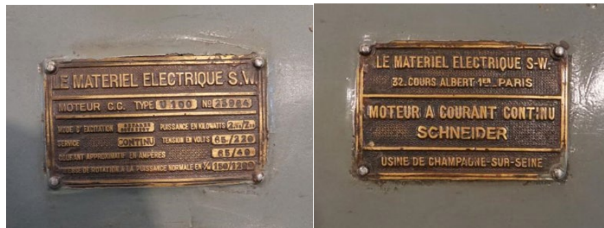
Figure 21. Motor Name Plate of the Electric Motor for the SOMUA Rifling Machine (Photo by author).
