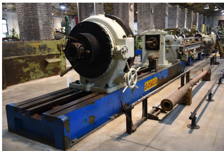
Figure 19. SOMUA Rifling Machine for Rifling the Barrel of the 36 Type Mountain Howitzer (Photo by LIU Guihong).
