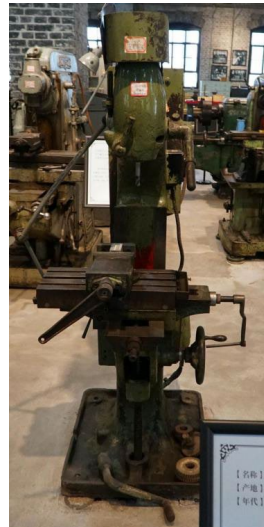
Figure 17. A vertical milling machine manufactured by NWIC in 1917.
