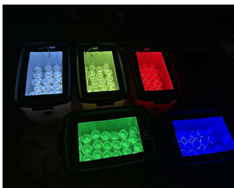
Figure 1. Exterior and interior views of the testing environment. Note. The six containers were used to each house 25 jars. Each jar contained one 2"L × 2"W × 2"H block of EPS and six Z. morio larvae. The container with the no visible light treatment is located to the right of the container with the red visible light treatment. Picture taken by Tyler Ferenz.
