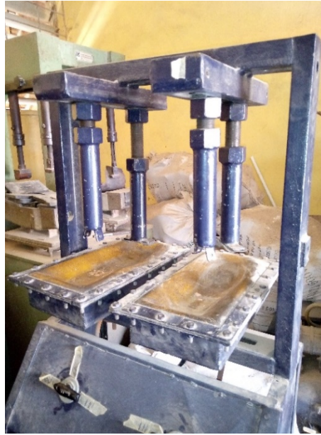
Figure 5. Footwear manual adjuster machine use for adjusting the sole of the shoe.
