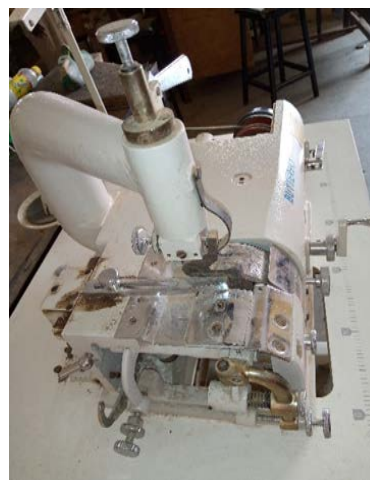
Figure 4. Picture of a bender machine use for bending leather fabric together.
