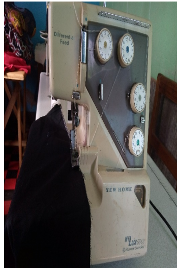
Figure 2. An overlock sewing machine used in finishing.
