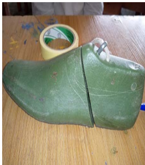
Figure 6. Foot last use for creating shoe design and lasting of the shoe.
