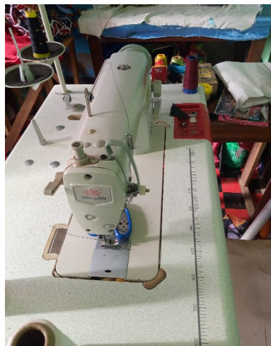
Figure 3. An industrial flatbed sewing machine used in joining two or more pieces of fabric together.
