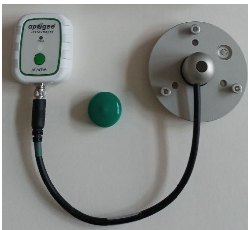
Figure 9. Apogee SL-510 upward-looking pyrgeometer with Bluetooth microcache datalogger.
